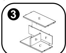
Take panel F, insert the dowels of panel F into the dowel holes of Panel C. Take Panel E, insert the dowels of panels D and F into the dowel holes of panel E to form "base." Lay base down on the back side of Panel F.
