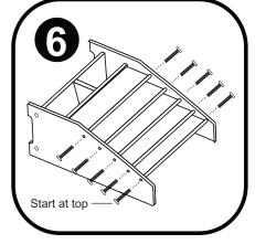
Bookshelf (minus slings) is now assembled on its back. With sling in hands, face tunnels towards you. Starting with the deepest sling pocket on top (care label is facing the floor on the backside of the top/deepest slng pocket), finger tighten hex bolts into each end of rods aligning top rod with top holes of panels A and B, continue down.
