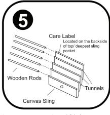
Lay canvas sling (G) flat on floor with tunnels facing up. Insert all wooden rods into canvas tunnels.
