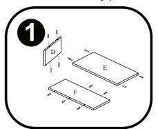
Insert all dowel rods into holes on the edges of panels D,E,F
