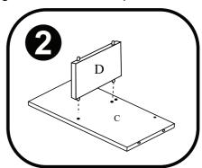
Take panel C (bottom base) face up and place the dowels of panel D into the center dowel holes on the face of panel C.
