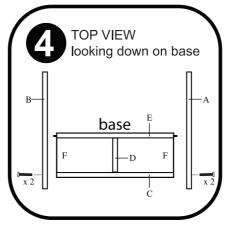
Align dowel holes of panel A to dowels of panel E. Finger tighten bolts into bottom holes of panel A, securing panel A to base. Align dowel holes of panel B to dowels of panel E. Finger tighten bolts into bottom holes of panel B, securing panel B to base.
